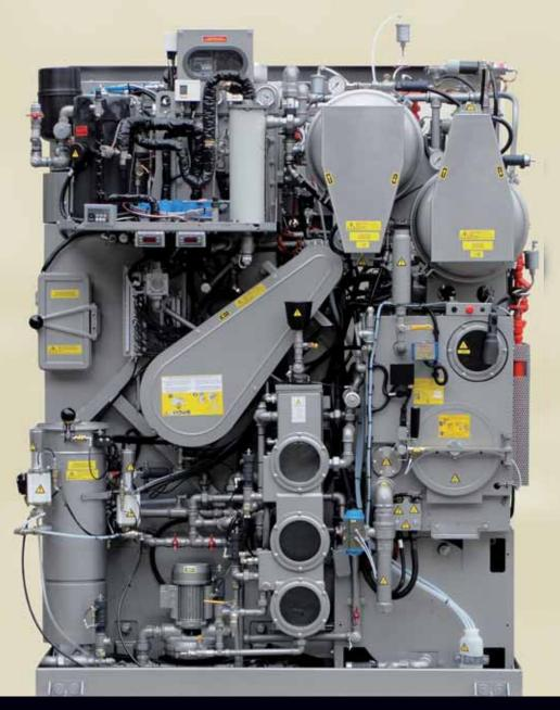
Logically and ergonomically designed for convenience; easy access to all maintainable components. This model includes multiple independent spin disc EcoFilters, carbon cartridge filters. There is convenient access to the generously sized double lint filters and button trap, the Multi-stage H.C.S. gravitational water separator with a large sight-glass.
