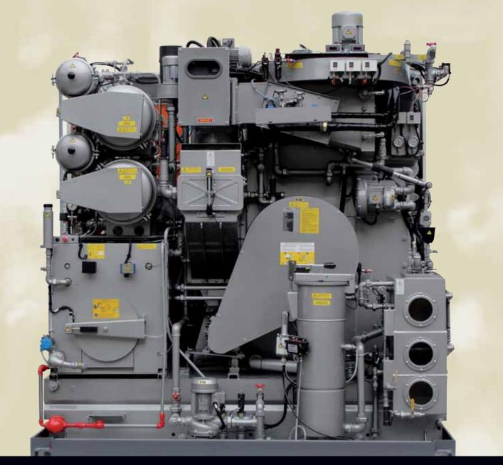
Logically and ergonomically designed for convenience; easy access to all components for quick maintenance. Multiple, independent spin disc EcoFilters® and carbon cartridge filters. Convenient access to oversized double lint filters and button trap. Extra-large fan and fridge unit. Multi-stage gravitational water separator with sight-glasses. Modular designed refrigeration system.
