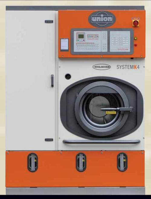
Exceptional cleaning, economy and ecological performance in 15 kg loading capacities. Two or three independent fully automatic tanks. Available in slim or cross line configuration. Large access aluminum loading door.
