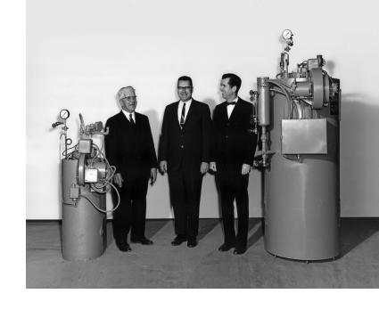
In 1949, Fulton pioneered the vertical tubeless design which quickly became the industry standard for industrial steam boilers. Since that time, no one has been able to improve upon Fulton's original design.
